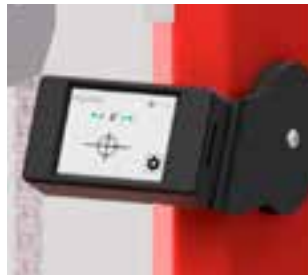
Touch screen. Log function. Possible to program e.g. several stops, turning angle, speed, rotation. Shows error messages.
