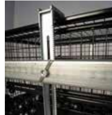
Box holders with or without clamps (optional extras) can be fitted. Clamps are recommended when tilting more than 60°.
