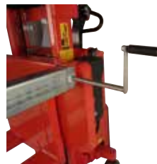
Adjustable box holders: The width is adjusted by a handle, so that the width fits the requested box width (between 800 mm and 1200 mm).
