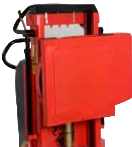
Multi-purpose carriage, which can be adjusted to fit specific customer items, e.g. tools.
